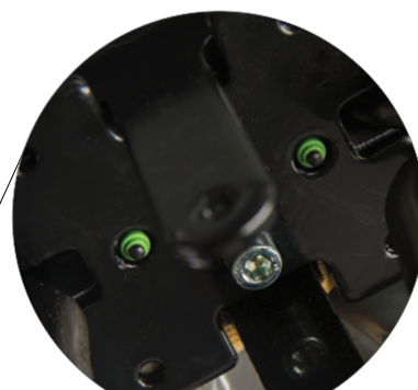
Upper and lower limit micro switch
